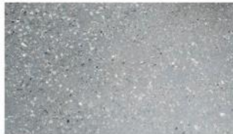
Upcycled concrete with aggregates of reused concrete.
