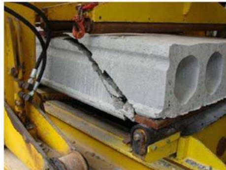
Real shear tension capacity at 20°C:  $V_{test} = 262 \text{ kN/slab}$
