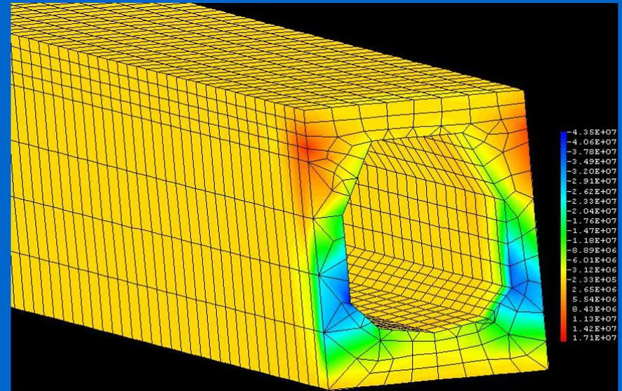
Shear by thermal strain
