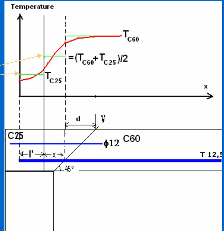
$$f'_{bpd,fi} = \eta_{p2} \eta_1 \frac{0,7 f_{ctm,C50} k_{c,t} \left( \frac{T_{C60} + T_{C25}}{2} \right)}{\gamma_{c,fi}}$$
