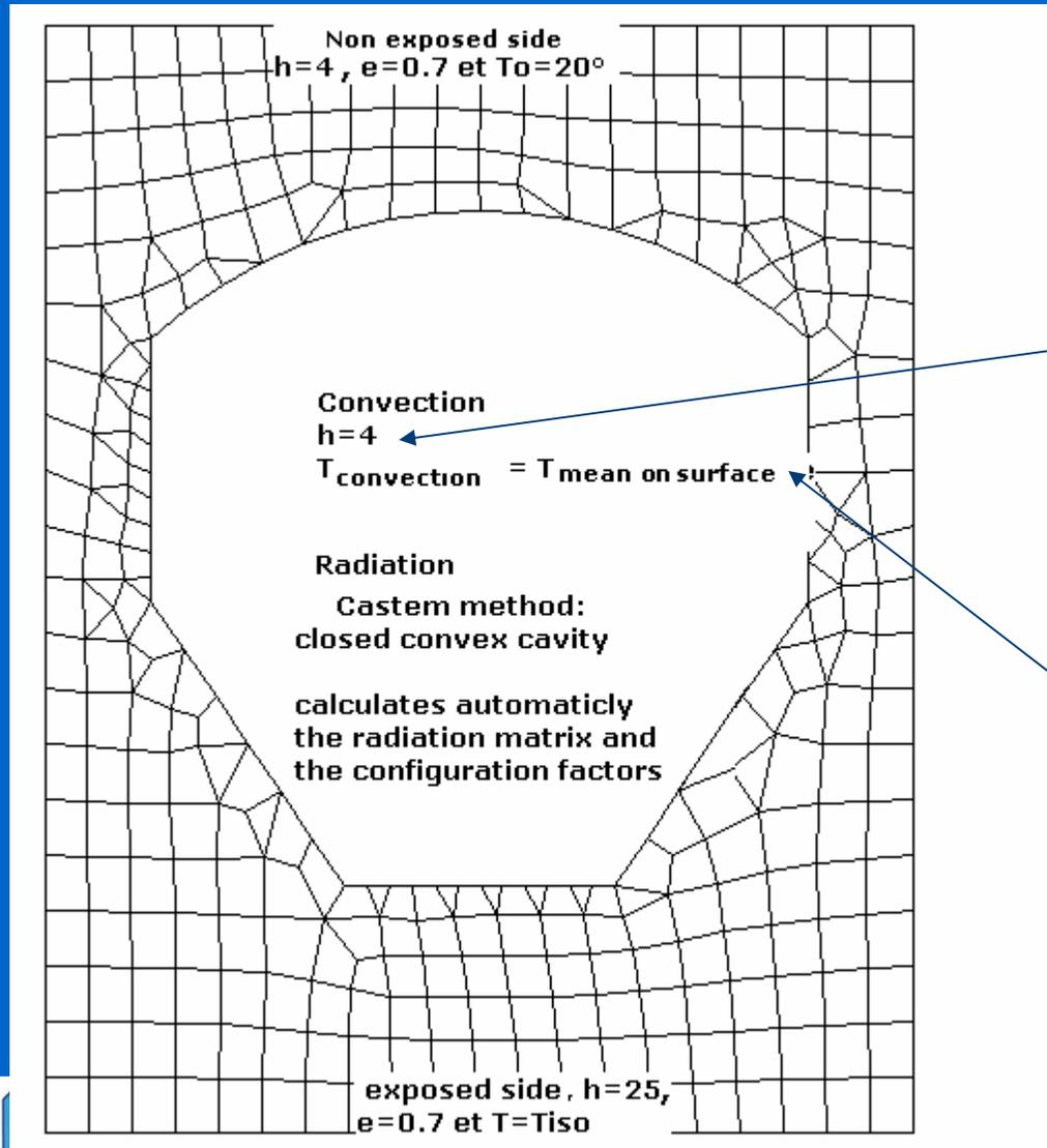
The convective heat transfer coefficient in the cavity is the same that for non exposed surface
