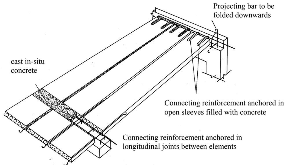
Fig. 13: Connections between hollow core floor and supporting structure
