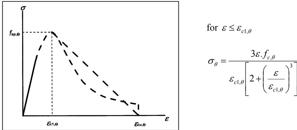
Fig. 8 Mathematical model for stress-strain relationships of concrete under compression at elevated temperature
