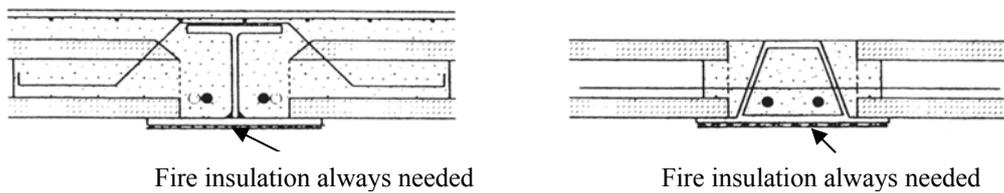
*Fig. 14: Examples of slim floor structures*
