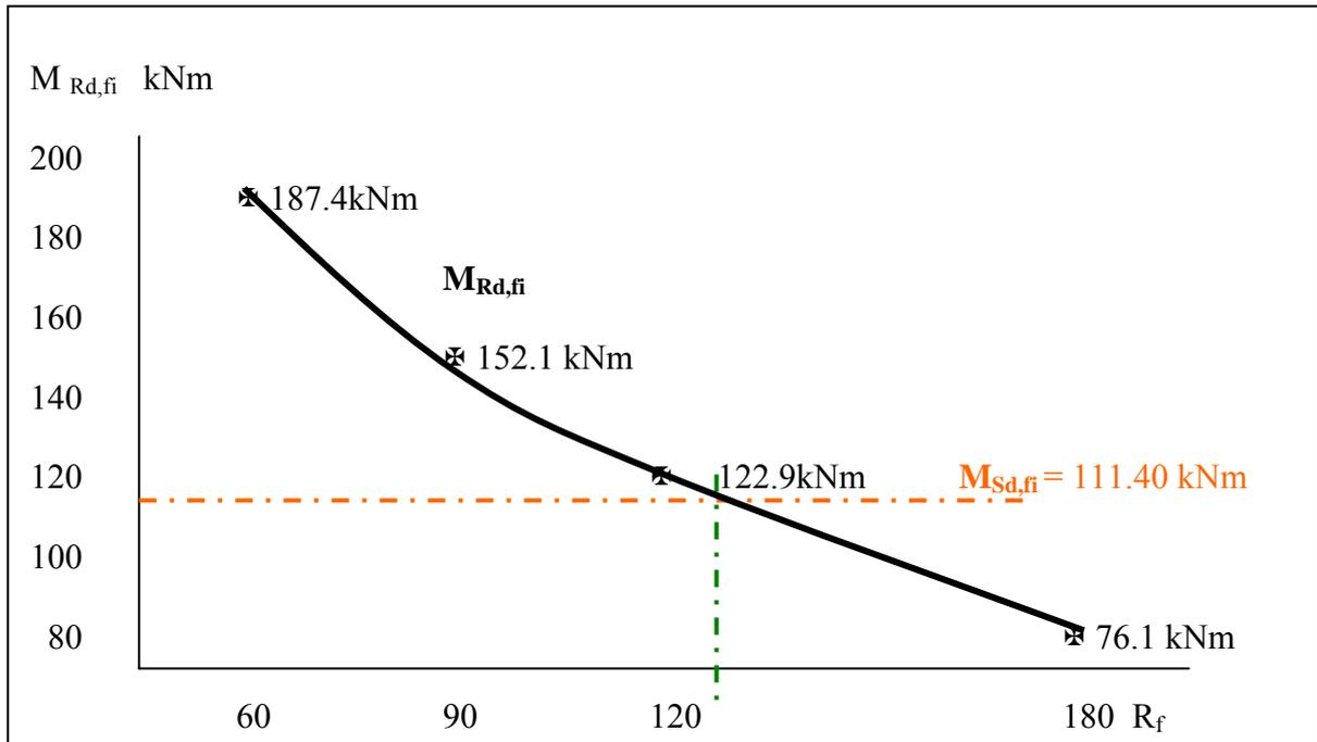
Fig. 4 Bending capacity at fire of a HC floor of 265 mm thickness
