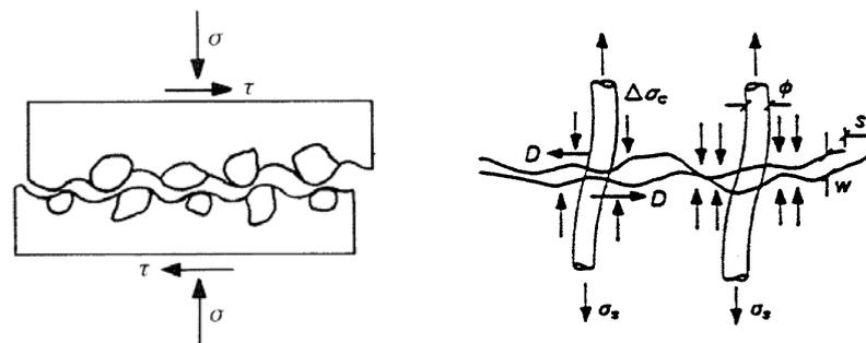
Fig. 12: Transfer of shear forces through aggregate interlocking
