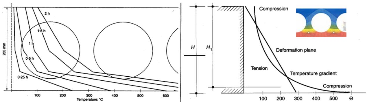
Fig. 10: Temperature profiles in a hollow core slab and induced stresses in the cross-section.
