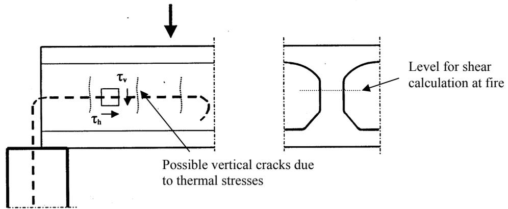
Fig. 11 Longitudinal section of HC under shear loading
