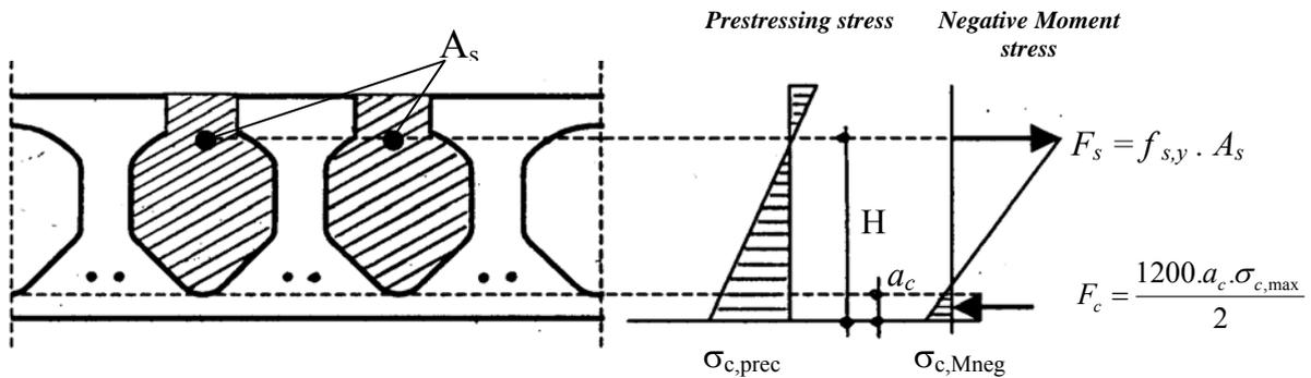
Fig. 9 Compressive stress of hollow core lower flange due to  $M_{neg}$  and prestressing
