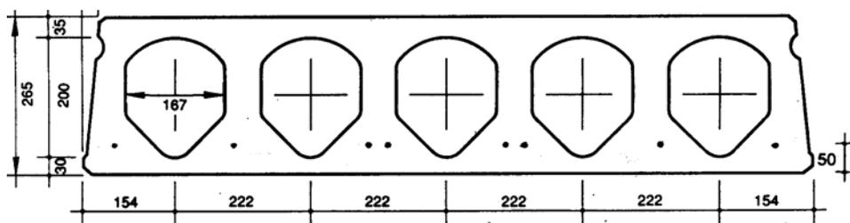
Fig. 2 Hollow core slab of 265 mm thickness
