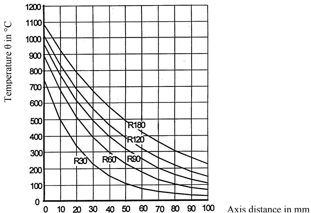
Fig.1 Temperature distribution in hollow core elements during standard ISO fire for siliceous aggregate concrete (Source EN 1192-1-2: Eurocode 2 Part 1-2: General rules – Structural fire design” [1])
