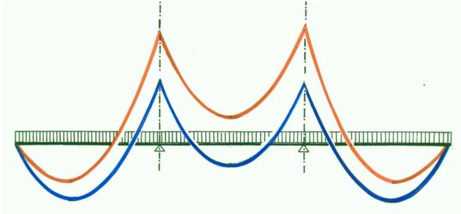
Fig. 6 Bending moment line in a continuous floor structure:
