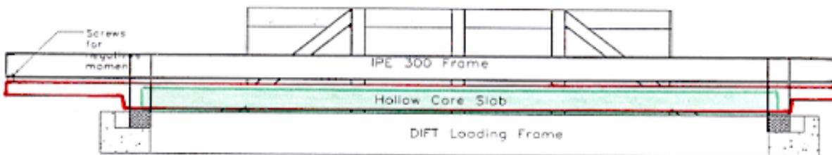
Fig. 7: Test set-up HC floor with restrained support
