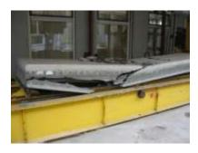
A260 12 Ø12,5 100 mm topping  $F_{exp} = 430 \text{ kN}$  $F_{calc} = 411 \text{ kN}$
