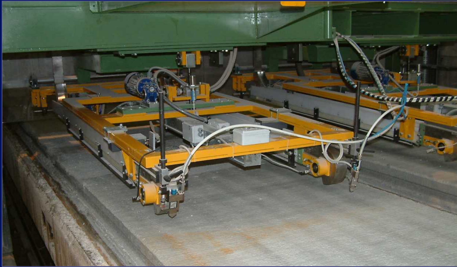
Card Applicator station with product passing underneath
