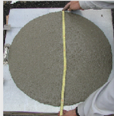
Consistency class S5/S6 & SCC Fluid Concrete
