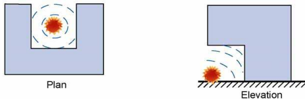
SHAPES THAT ACCENTUATE AIR BLAST
