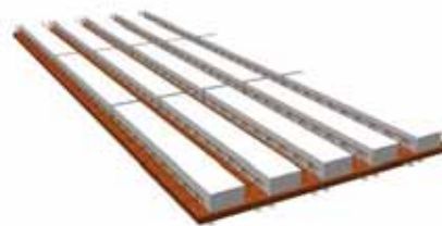
Brick Floor with Fill
