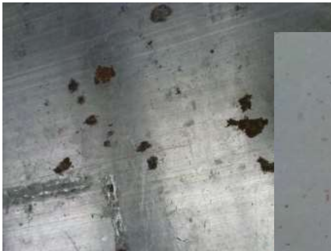
Reference situation: Corrosion on the form
