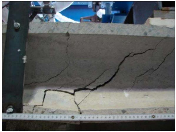
Shear failure Series G
