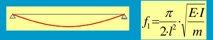
More accurate determination of frequency possible if requested (dynamic analysis, FEM) – but input data should be determined as accurate as possible!
